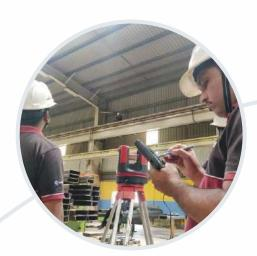
For safe and smooth operation of your cranes, perfect levels, track straightness and parallelism of the tracks are extremely important. Tracks ensure longer life and safe operations of cranes and their components.
